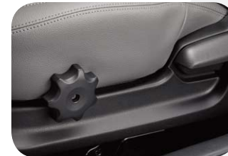
Driver's seat cushion tilt adjuster
